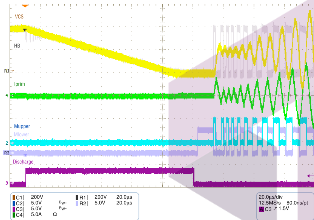
Figure 48. Initial Resonant Capacitor Discharge before Dedicated Startup Sequence is Placed
